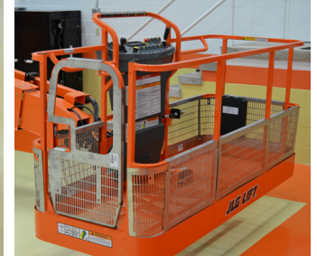
Mesh to Mid Rail
