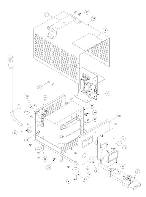
Its simple method of operation and trouble-free performance makes it attractive to use. To operate, after the charger is connected to AC power, simply plug in the DC cord set to activate the unit. The charger then automatically charges the battery, and also monitors the battery condition determining the proper charge profile and the correct finish phase before automatically terminating the charge when the battery is fully charged.
