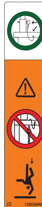
SJ126056 Falling Hazard
